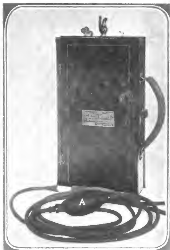
Fig. 5—View of the instrument when not in use. It is of first importance to remember that the cock should then be closed, and the plug be used to seal up the rubber tube above CO 2 chamber, lest disastrous results are the expectation.
